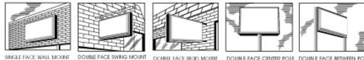
SINGLE FACE WALL MOUNT DOUBLE FACE SWING MOUNT DOUBLE FACE KNOB MOUNT DOUBLE FACE CENTER POLE DOUBLE FACE BETWEEN POLE
